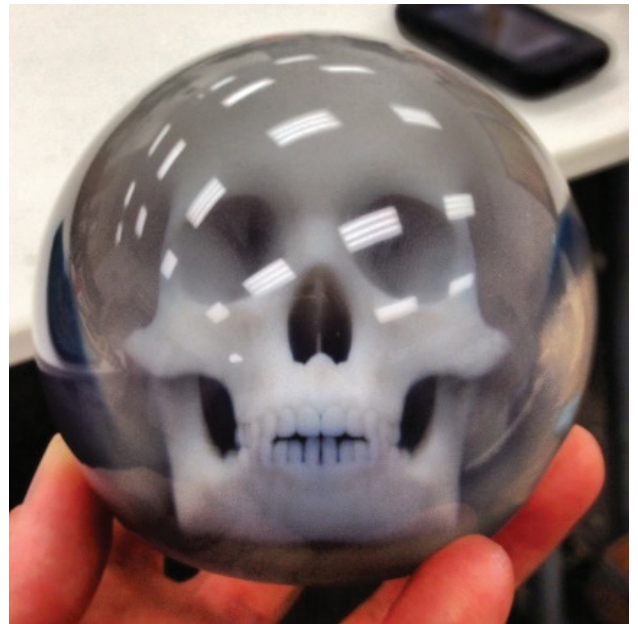
Figure 17: The effect of polishing on transparent and translucent parts.
