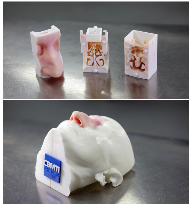
Figure 13: Consumable models like the nasal cavity (top) can be placed in a reusable fixture (head model, bottom).
