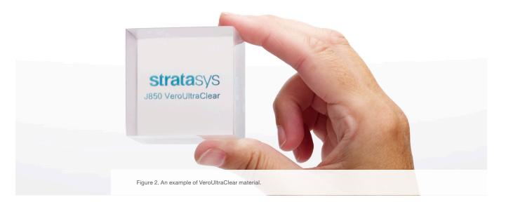
PolyJet technology offers three rigid materials that provide either translucency or transparency, RGD720, VeroClear<sup>™</sup> and VeroUltraClear<sup>™</sup>. VeroClear and VeroUltraClear have the same properties as the rest of the Vero family, and RGD720 is also strong and stiff.
