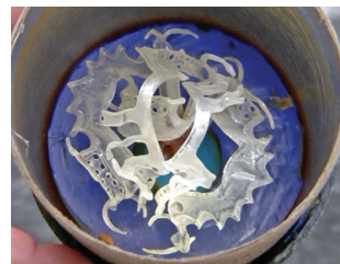
Figure 7: A coated cardboard casting ring and multiple partial framework patterns attached to the base.
