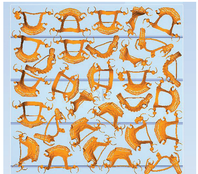
Figure 3: A build tray with RPD patterns.
