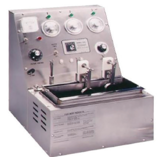
Figure 16: Place the partial plate framework in an electrolytic de-plating machine such as this Esmadent Electropolisher.
