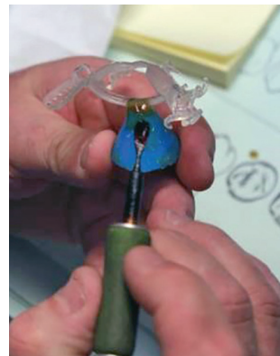
Figure 6: Attaching the sprue of the partial plate to the base former.
