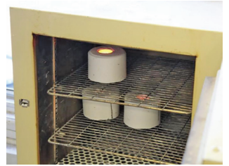
Figure 14: Cast rings cooling on the cooling racks.
