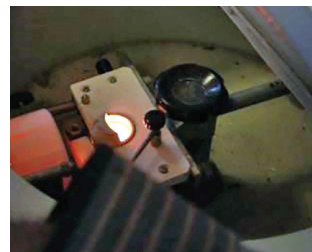
Figure 13: Place the casting ring into an induction casting machine.
