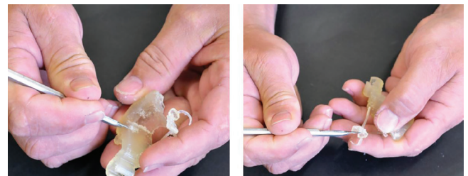
Figure 4: Mechanically remove the soluble support from the 3D printed partial plate framework pattern.
