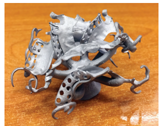
Figure 17: Multiple frames produced in a single casting process.
