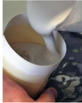
Figure 10: Pour the investment mix into the casting ring.
