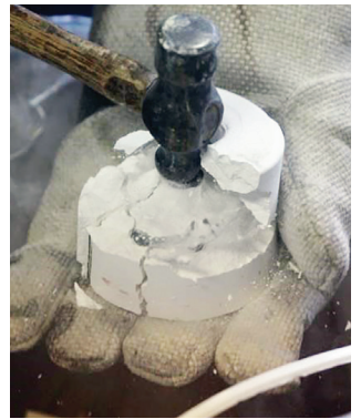
Figure 15: Break the investment surrounding the cast framework.
