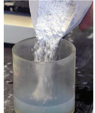
Figure 8: Combine the CADVEST investment powder and liquid.
