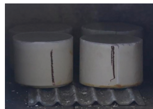
Figure 12: Casting rings inside the burnout furnace.
