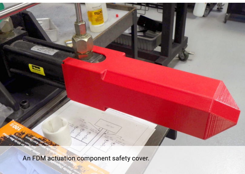
An FDM 3D printed protective cover.
