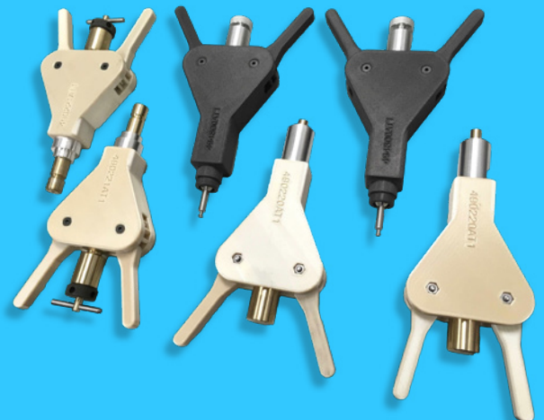
Puller tools incorporating integral identification labels
