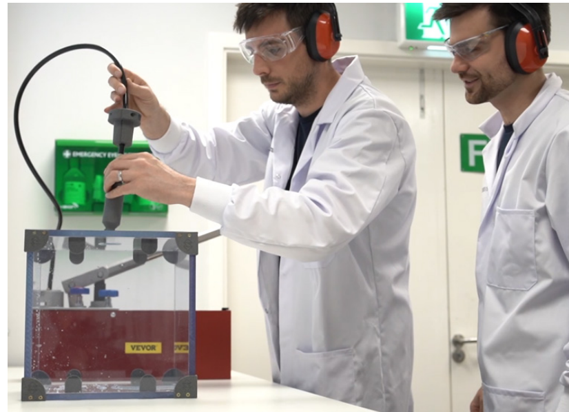
Figure 2: Cylinder being lowered into test chamber
